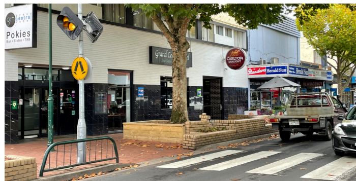
Zebra crossing with flashing beacon on Gray Street
