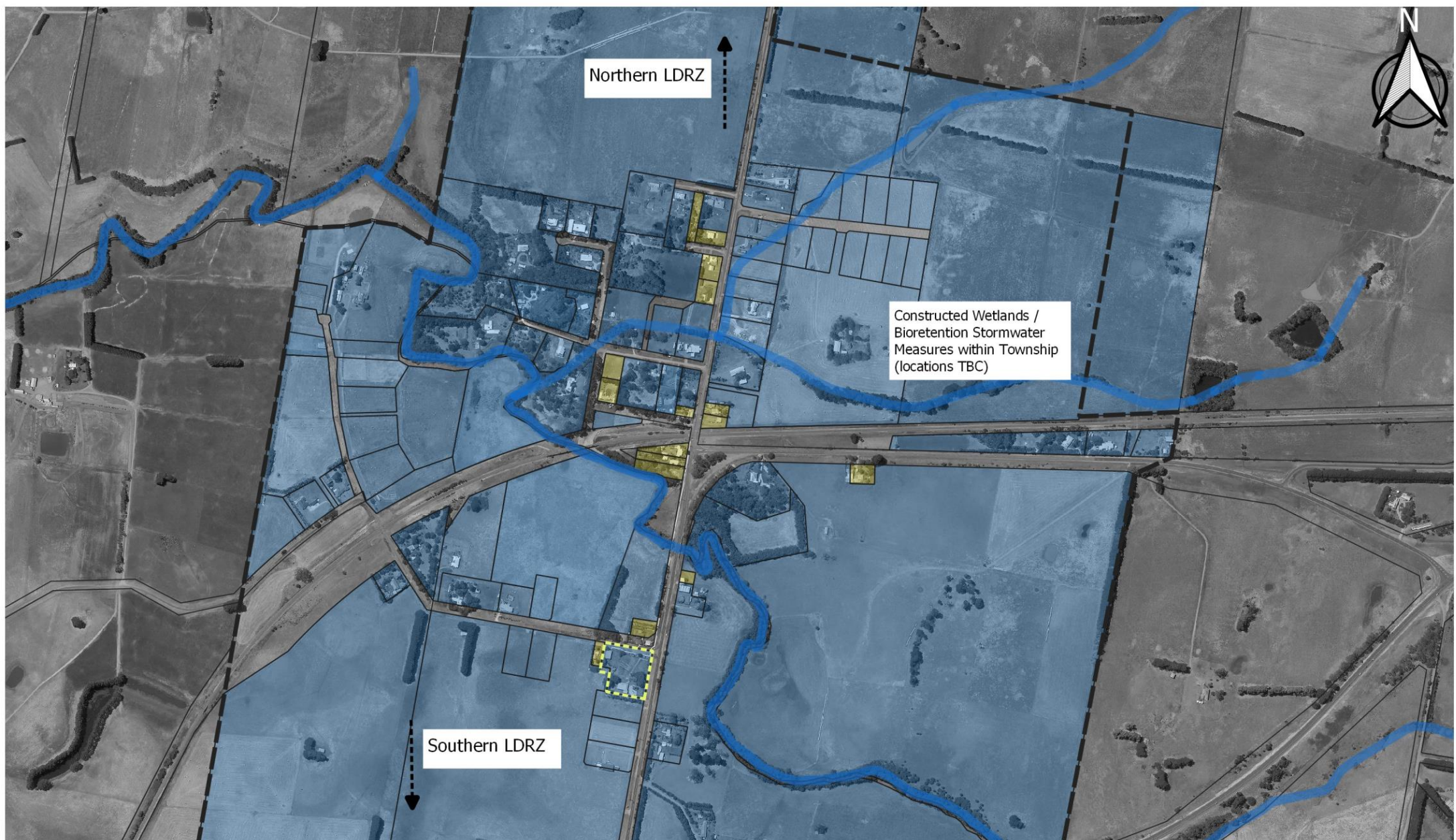
Figure 7: Cudgee Solution Package 2 Servicing Layout - Retain On-site Systems and Build Stormwater Treatment / Detention Measures
