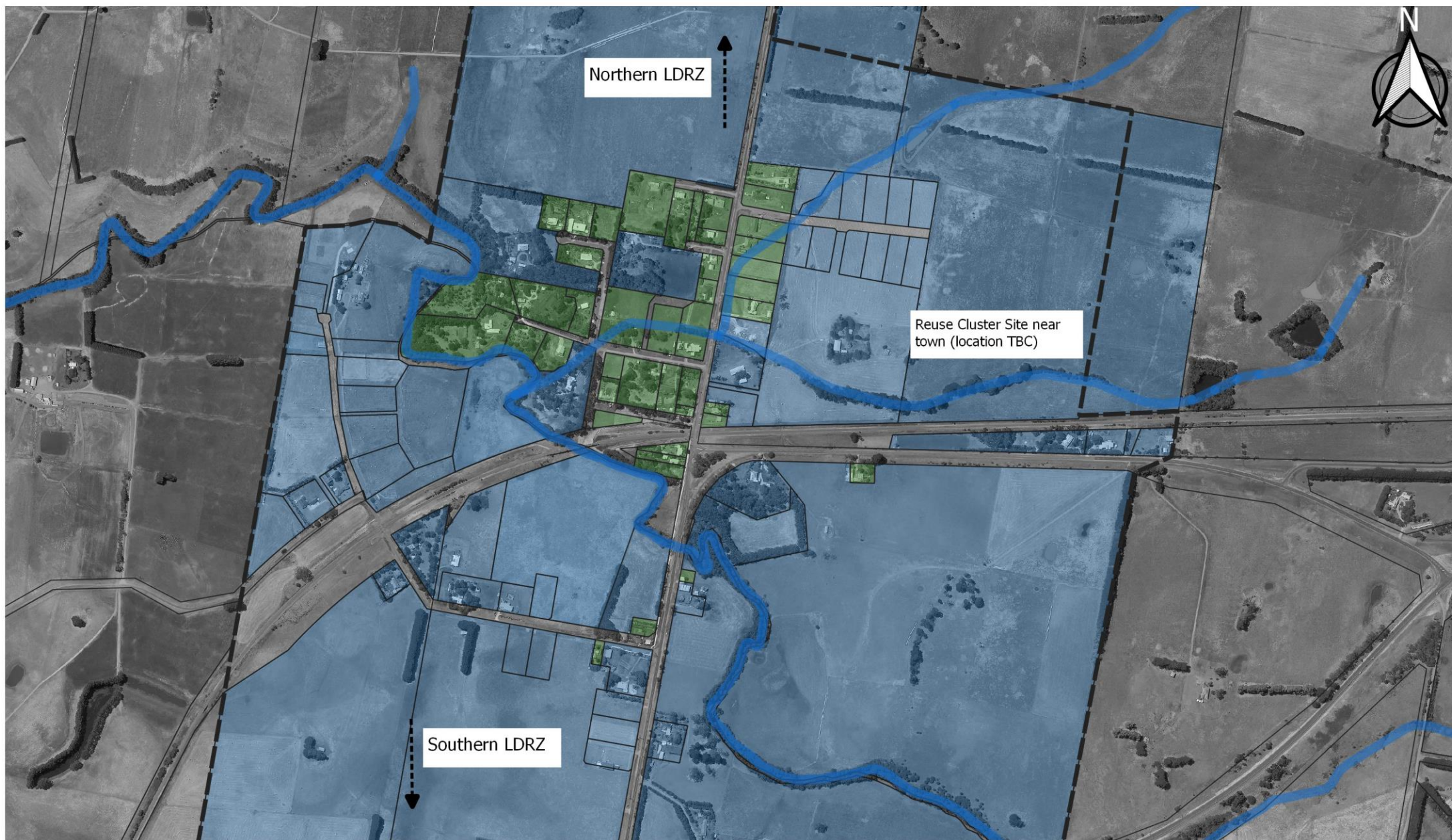
Figure 8: Cudjee Solution Package 3 Servicing Layout - Partial On-site Containment / Reuse with Cluster Irrigation Site
